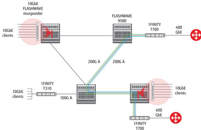
At the other end of the circuit, the two wavelengths are inverse multiplexed (i.e. re-combined) back to a single client signal. The 1 FINITY T700 is a carrier-grade, high port density solution (see Table 2) for 100/400GbE services that supports up to 20 client ports, 4 line ports, and a total switching capacity of 1.6T.
